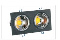
Lamp Parameters : Super-bright Standard Input Voltage AC100-277V or AC200V-240V Freqency Range 50Hz∼60Hz Led Consumption 40W System Consumption 45W Led Initial Flux 3300LM-3800LM 4400LM-5200LM Color Rendering Index >80 Working Temperature -40℃ ~ +55℃ V0 Fireproof Class 2x0.75mm2 Power cable Color of housing black, white, silver CE ROHS ERP V0 FCC Certificate Optical data: IES
