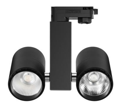
Two different reflectors are availble for the double head light, so that it can meet different beam angle requirements in the same area. As the above picture shown, the left is  $38^\circ$  beam angle while the right one is  $20^\circ$ .
